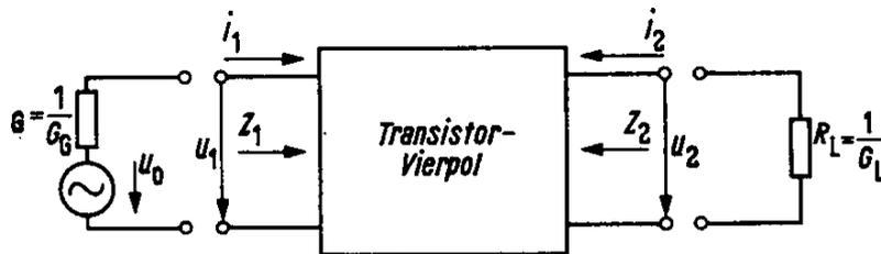
$$\text{Eingangswiderstand} \quad Z_1 = \frac{u_1}{i_1} = \frac{1 + y_{22} \cdot R_L}{y_{11} + \Delta y \cdot R_L}$$
