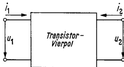
$$\begin{aligned} y_{11} &= g_{11} + jb_{11} \\ y_{12} &= g_{12} + jb_{12} \\ y_{21} &= g_{21} + jb_{21} \\ y_{22} &= g_{22} + jb_{22} \end{aligned}$$
